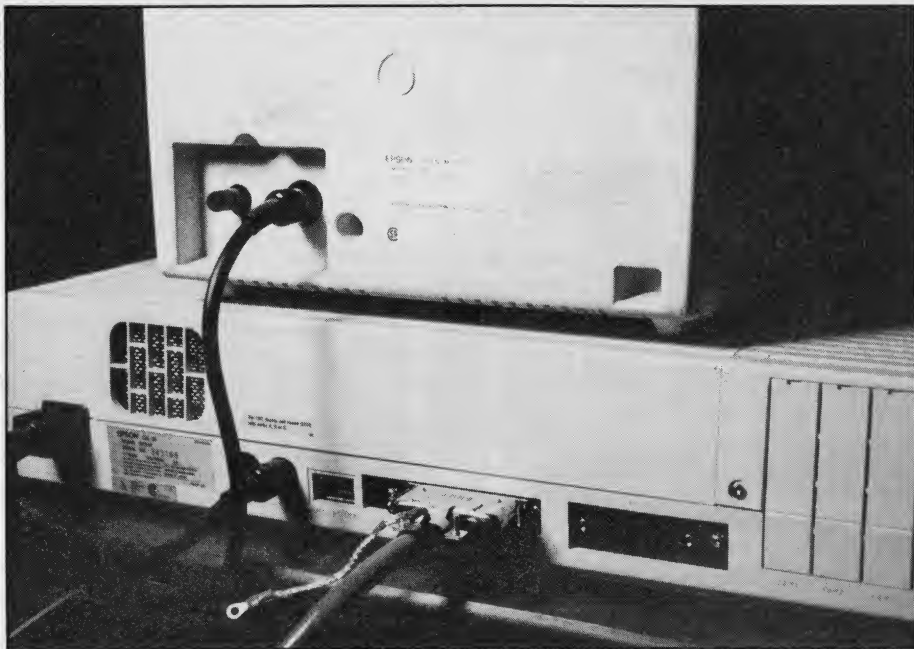
Rear of the system unit has connectors for parallel printer, RS-232 device, monitor, and AC power cord.
